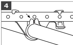
Note: The ears of the clamp should lock on the front of the bracket.
