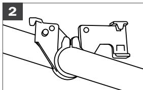
Insert tube into SimpleStrap clamp.
