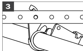
Align tooth through one of the bracket holes, twist clamp counterclockwise, and click tabs onto bracket.
