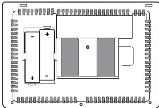
**NOTE:** We recommend replacing the thermostat batteries annually or if the thermostat will be unattended for an extended period of time.
