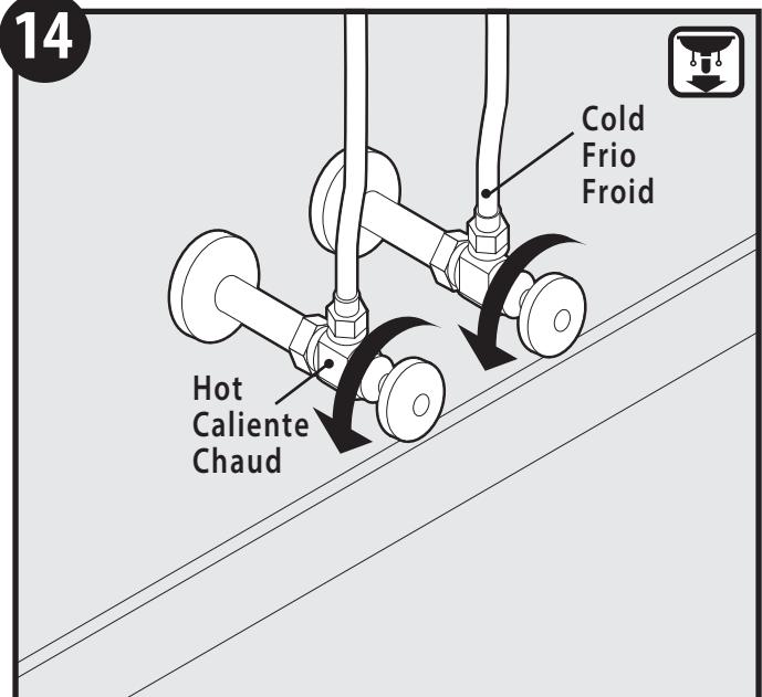
Attach other ends of Flexible Supply Lines (not included) to shut off stops. Tighten with wrench. Turn on water and check for leaks.
