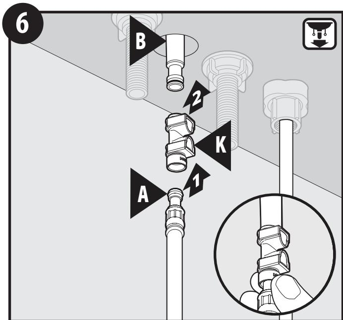
1) Install Side Spray (A) Hose into Quick Connect Adaptor (K). Push in as far as possible till a click is heard. Tug downward to test engagement.
