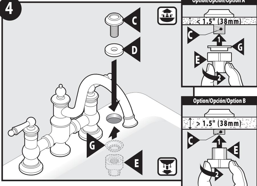
For "Thin Deck" applications, countertop and sink thickness less than 1/2", install Nut (G) and Hose Guide (C) onto the Hose Guide Mounting Nut (E). Thread on Hose Guide Mounting Nut (E) by hand.
