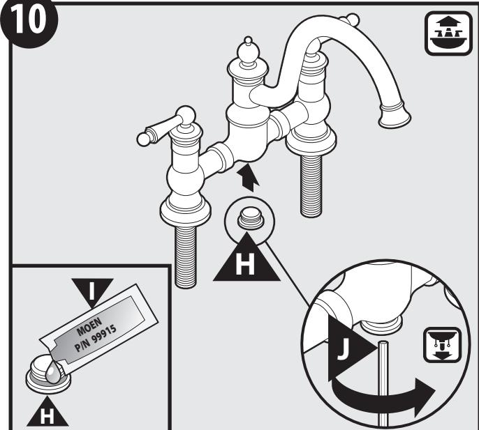
Apply a small amount of Lubricant (I) to Hardware Plug (H). Insert into bottom of Faucet Body (B). Secure with Hex Wrench (J).
