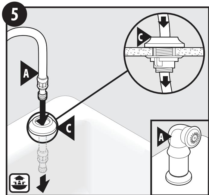
Insert Side Spray (A) into Hose Guide (C) until Side Spray is fully seated.
