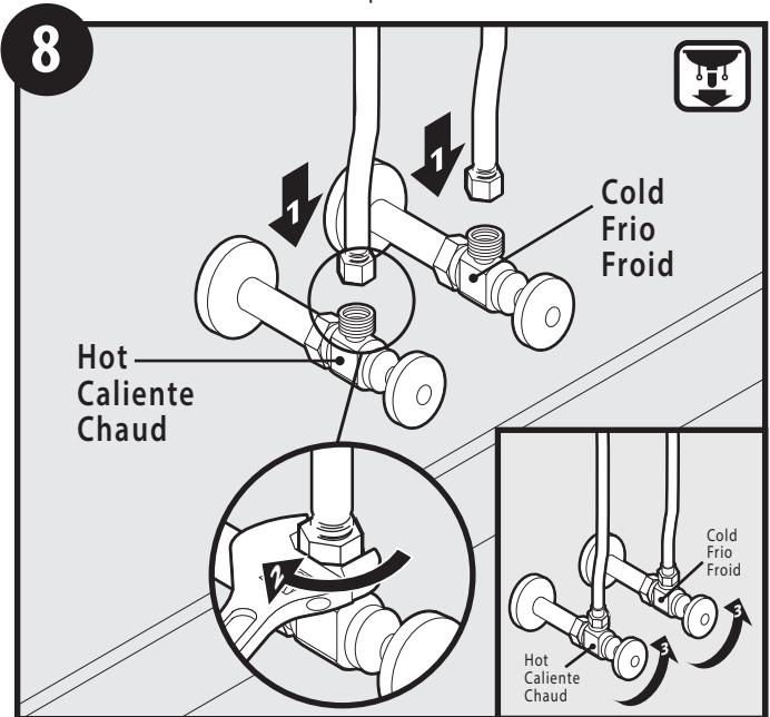
Attach other ends of Flexible Supply Lines (not included) to shut off stops. Tighten with wrench. Turn on water and check for leaks.
