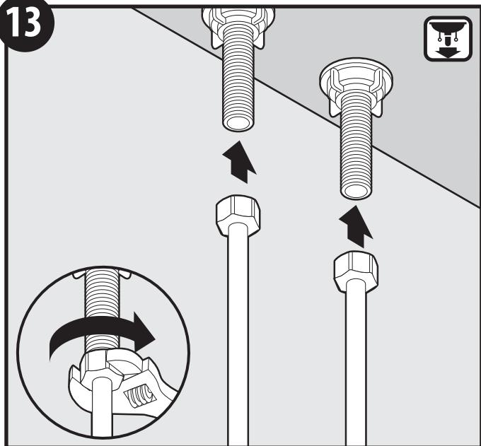
Attach Flexible Supply Lines (not included) to Faucet Body (B) shanks. Secure with wrench.
