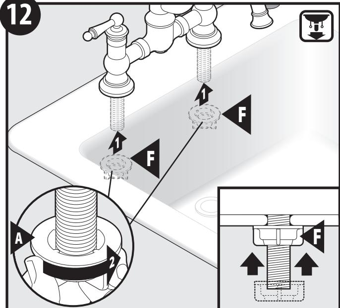
Install Mounting Nuts (F) onto Faucet Body (B) shanks and tighten firmly by hand.
