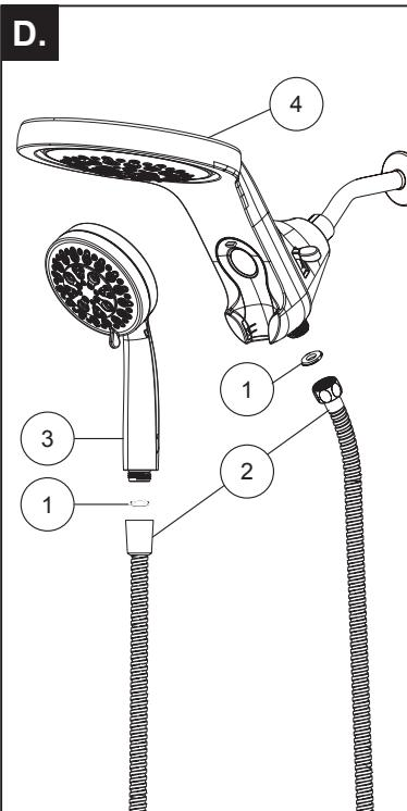
Place the hose gaskets (1) into the hose nuts on each end of the hose (2). Connect one end of the hose to the shower head (3) and the other end to the hand shower (4). All connections should be able to be made by hand tightening.
