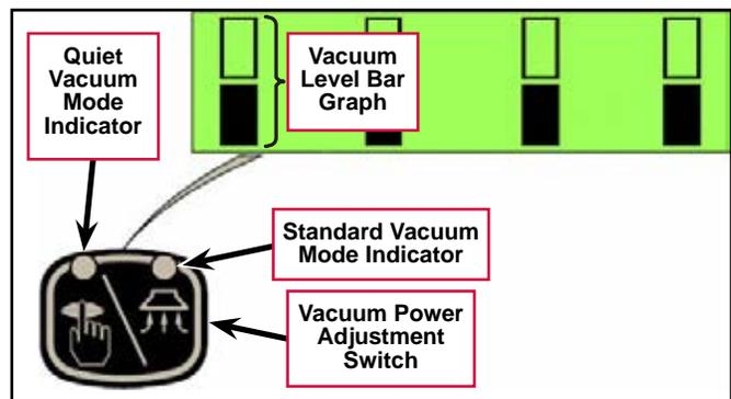
Pressing the **Vacuum Power Adjustment Switch** during this 10-second delay period will shut off the vacuum motor immediately.
