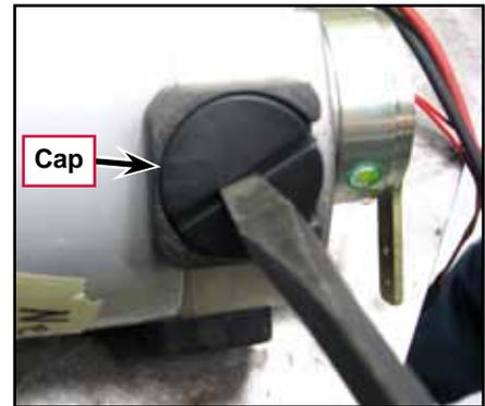
4. Carefully pry out the old Brush from the motor.
