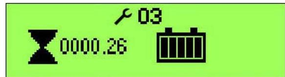
If more than one fault exists, the display will sequence through the fault codes at one-second intervals. If the error is significant and results in a machine system shutdown, the graphic display will show the Information Screen until next key switch cycle. Otherwise the Information Screen will be active only when the Information Switch is pressed.
