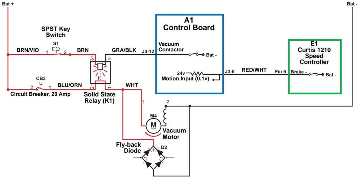
The following conditions must be met before the **Vacuum Motor** can start:
