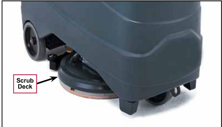
The **Scrub Deck Motor** is mounted on the top of the **Scrub Deck**. Note that the 20D Scrub Deck and Brush Motor are shown here.
