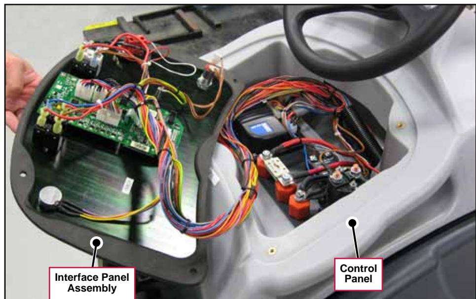
4. Carefully disconnect the **Electrical Connectors** from the **A1 Control Board**.
