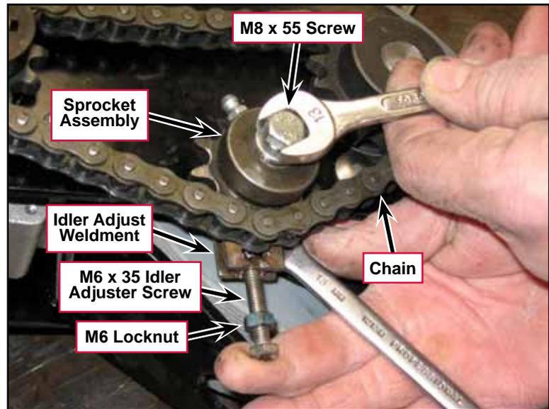
5. Remove the **Master Link** and remove the chain.
