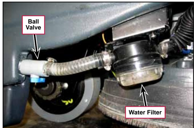
The **90° Ball Valve** and **Drain Hose** allow you to drain the solution tank.
