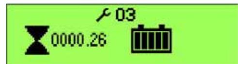
When the **03** is displayed, the Detergent On/Off Indicator will flash a special error code sequence until the fault is corrected. (The Forward/Reverse LED may also flash on some models.) See the [“Status LED Fault Code Table”](#) on page 122 for a description of the fault indications.
