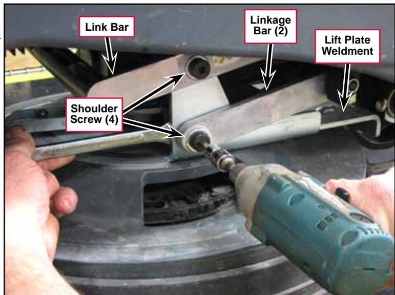
11. Remove the **Shoulder Screw** and nut that connect the scrub deck actuator to the **Lift Plate Weldment** on the scrub deck. Note that you'll need to hold the M8 Nyloc® nut with a 13mm wrench while you remove the **Shoulder Screw**.
