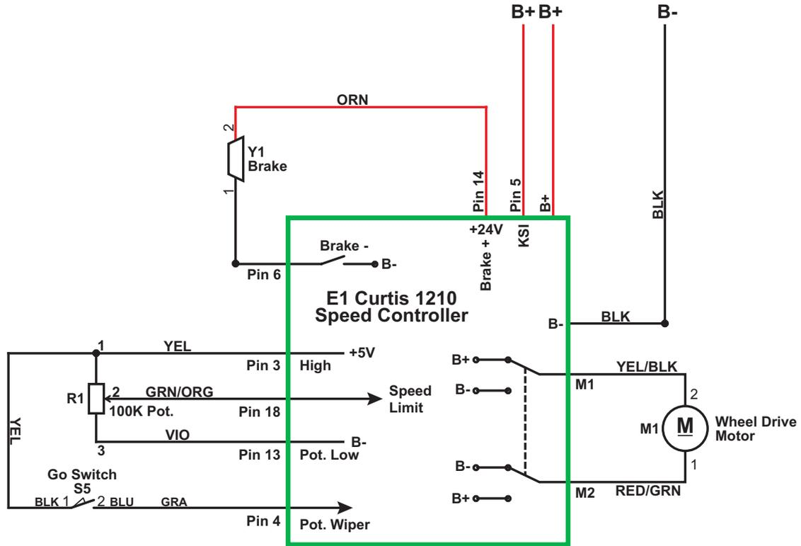
The **E1 Curtis 1210 Speed Controller** provides a regulated 5-volt supply out **Pin 3 - High** to the **100K Pot.** (speed potentiometer) and the **Go Switch S5**. When the Operator steps on the Go Pedal, the **Go Switch** closes and sends the 5 volts back to **Pin 4 - Pot. Wiper** on the **Speed Controller**.
