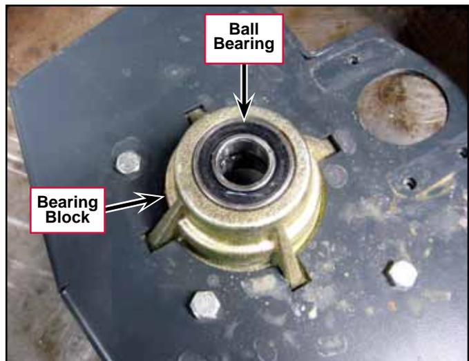
9. Reassemble the Drive Wheel Assembly by following the above steps in reverse order. Note that when you reinstall the 1"-14 Nyloc® Nut onto the Spindle Weldment, torque the Nut to 20 ft.-lbs.
