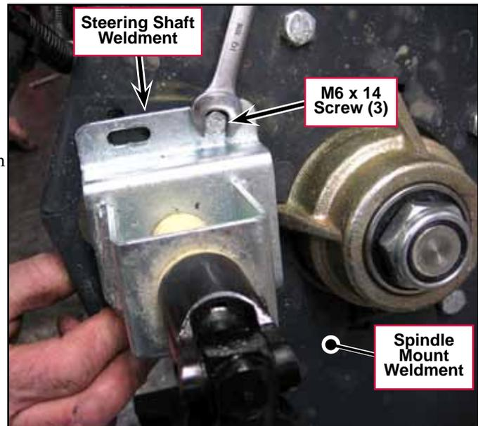
5. Remove the 1"-14 Nyloc® Nut from the Spindle Weldment.
