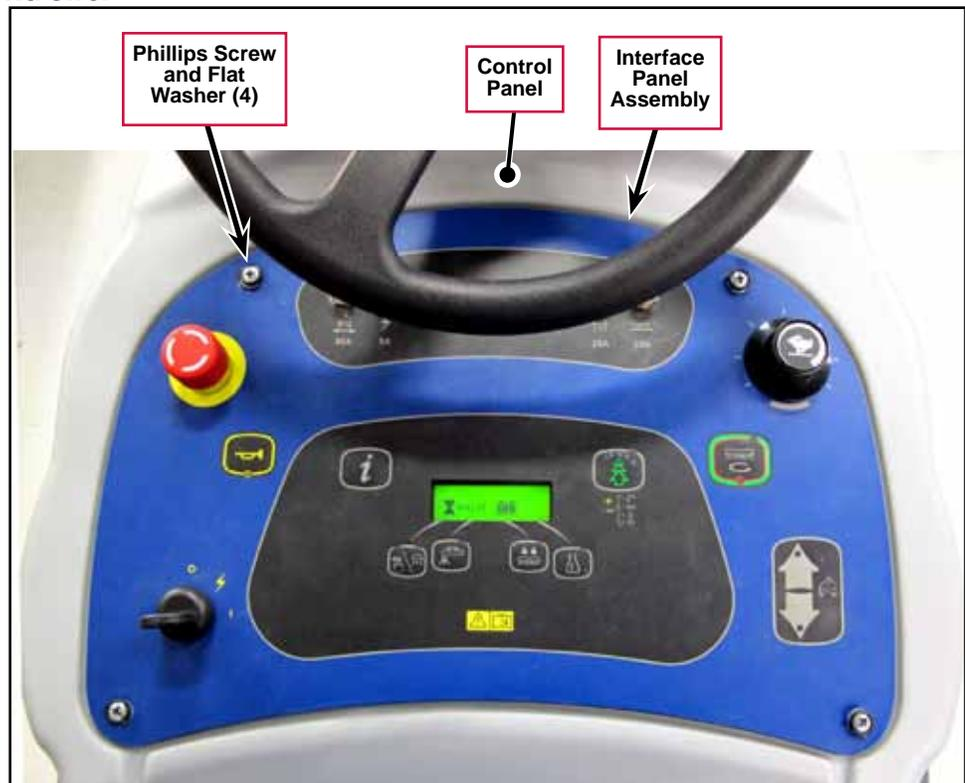
3. Carefully lift the **Interface Panel Assembly** out of the **Control Panel**.
