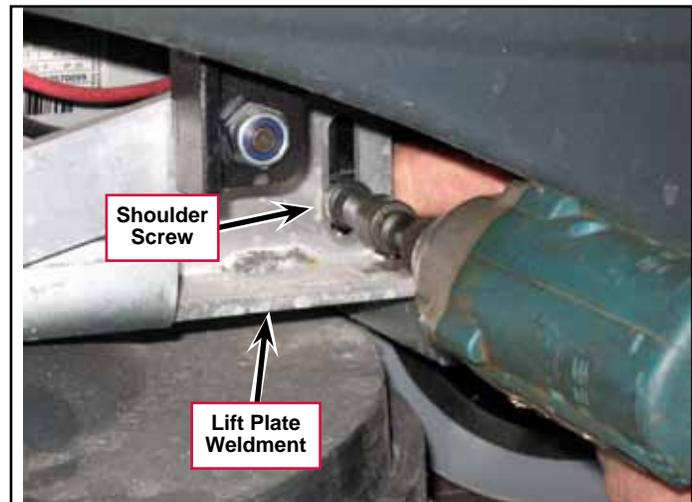
6. Remove the **M10 Screw** and actuator spacer holding the **Scrub Deck Actuator** to the **Actuator Bracket** on the machine frame.
