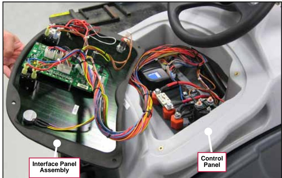
4. Carefully disconnect the **Electrical Connectors** from the **E1 Curtis 1210 Speed Controller**.
