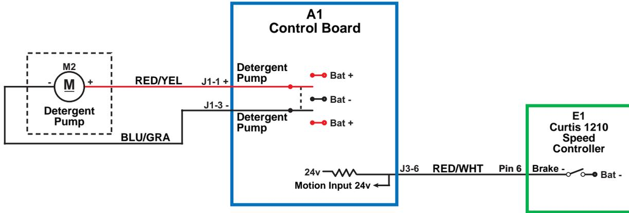
When the Detergent System is off, the **Detergent Pump** switches on pins **J1-1** and **J1-3** do not provide power to the **Detergent Pump**.
