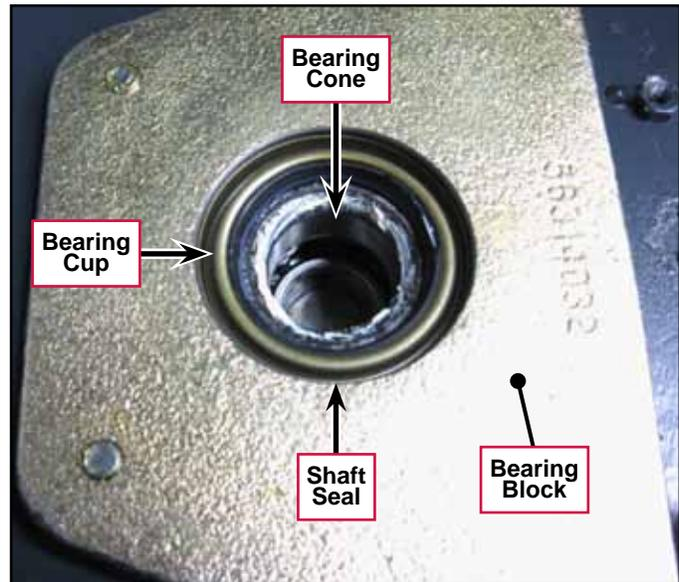
8. Remove and replace the Ball Bearing as necessary.
