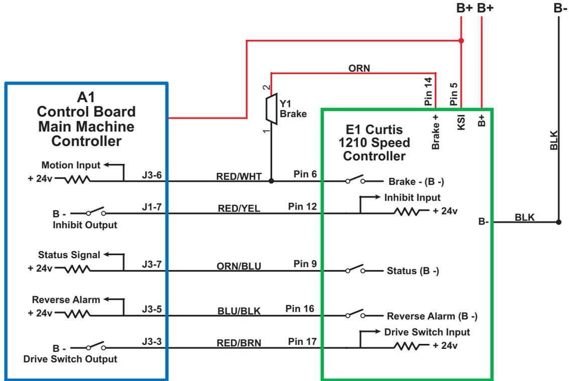
There are five “communication” wires that run between the **A1 Control Board** and the **E1 Curtis 1210 Speed Controller**. Each wire is used to communicate a unique piece of information as listed in the following table.
