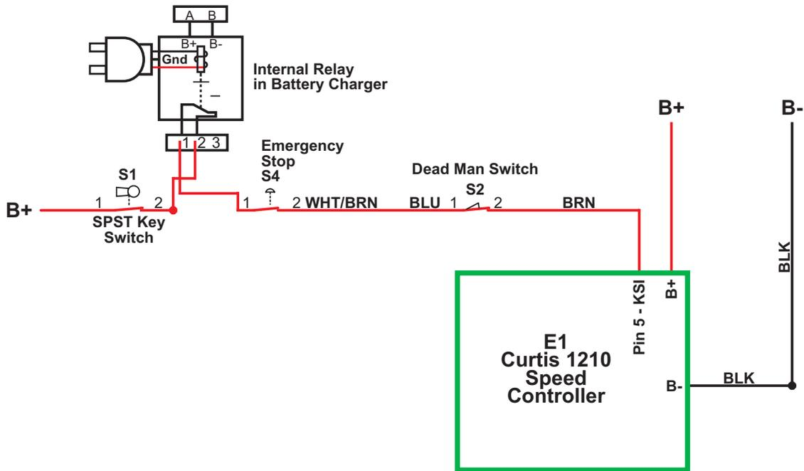
In order for positive voltage from the **SPST Key Switch** to reach **Pin 5 - KSI** (key switch input) on the **E1 Curtis 1210 Speed Controller**:
