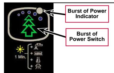
If any one of the functions listed above is already performing at its maximum possible rate, the **Burst of Power Switch** will have no effect on that function but will still affect the other functions. If the detergent option is not installed, the Burst of Power will not affect detergent flow but will still affect the other functions.
