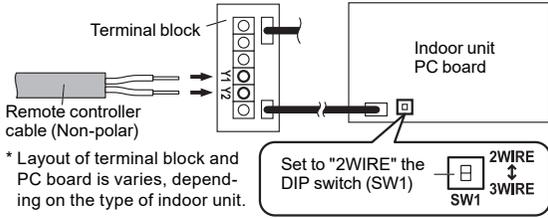
\* Layout of terminal block and PC board is varies, depending on the type of indoor unit.
