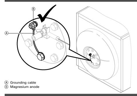
Check proper connection of grounding cable at magnesium anode.
