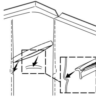
**22 STORE+® models only:** Seat the shelf on one side and back notch. Rotate into place.
