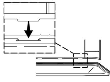
**13** Measure, mark, and drill the faucet holes in the drain end wall.
