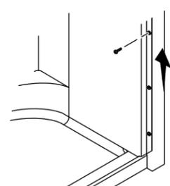
**17** Secure the walls to the studs along the top. Use shims as needed.
