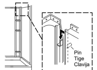
**15** The front edges should be flush, with no more than a 1/32" (1 mm) gap.
