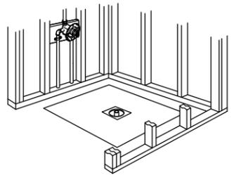
**5** Without a pad, we recommend the basin area be set in 1" (25 mm) to 2" (51 mm) of mortar cement.
