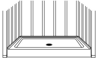
**7** With the unit level, shim under the support feet as needed.
