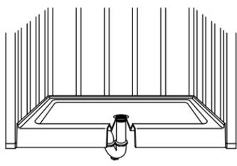
**10 Custom Walls:** Cut the finished wall as shown. Leave the weep channel open.
