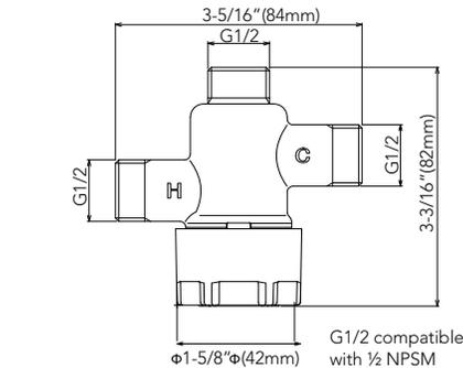
Thermostatic Mixing Valve (TLT10)
