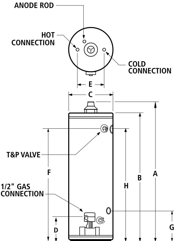
Maximum Hydrostatic Working Pressure: 150 PSI
