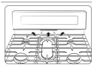
The oven vent is located under the oven Control panel. Proper air circulation prevents oven burner combustion problems and ensures good performance.
