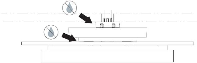
With water flowing through the showerhead, verify that there are no leaks.
