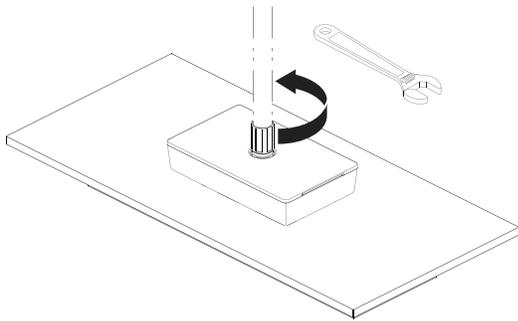
Install the showerhead onto the shower arm. Do not over tighten. **NOTICE: Removal of or tampering with the flow restrictor may result in showerhead failure and will void the warranty.**
