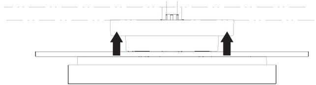
Gently release the escutcheon by pushing it up away from the showerhead to allow it to press against the ceiling.
