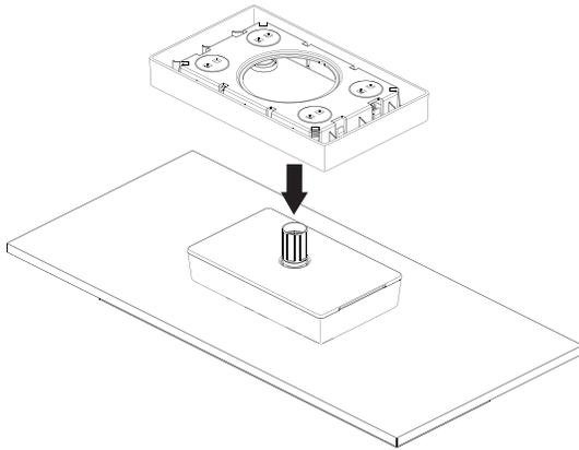
Install the escutcheon onto the back of the showerhead until there is a "CLICK" and the escutcheon remains compressed.
