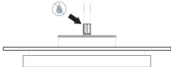
With water flowing through the showerhead, verify that there are no leaks.
