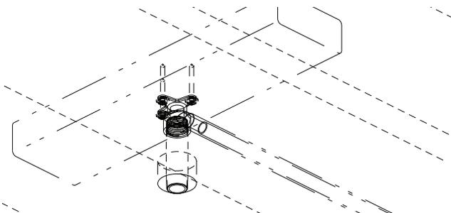
For all installations, the supply line must be secure and be able to support 15 lbs. (7 kg) of weight.
