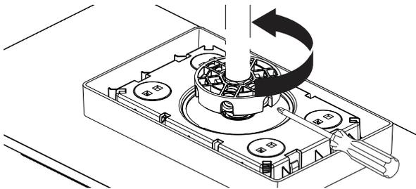
Install the shower head onto the 1/2-14 NPT fitting. Use a screw driver to turn the installation tool. Do not over tighten. **Notice: Removal of or tampering with the flow restrictor may result in shower head failure and will void the warranty.**
