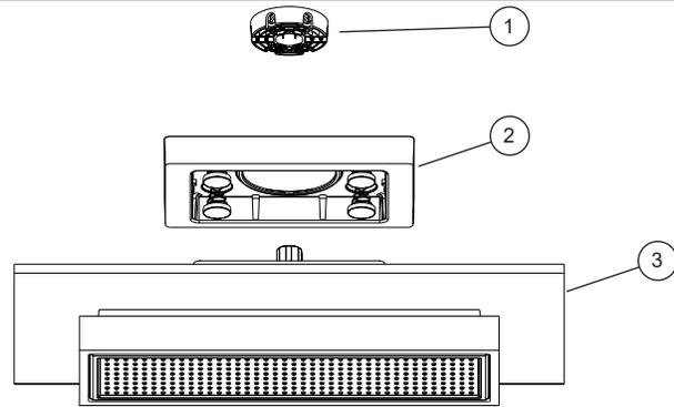
For pendant mount installations on a vertical shower arm, the surface mount installation tool and escutcheon can be removed and discarded.
