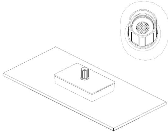
Verify that the filter gasket is installed in the female nut on the showerhead.
