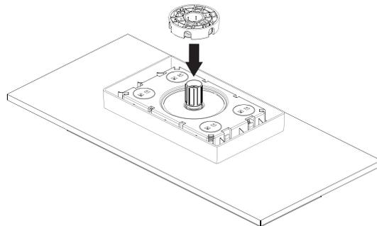
Install the installation tool onto the showerhead ball joint.
