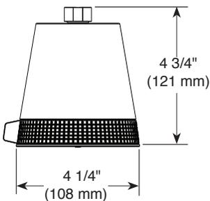
52668▲ 1.75 GPM 5-Function Shower Head w/H<sub>2</sub>Okinetic® Technology
