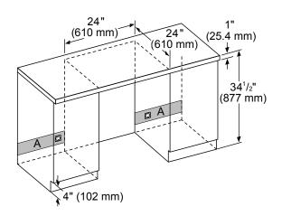
Recommended area for installation connection - a 2<sup>1</sup>/<sub>2</sub>" (63 mm) diameter hole is recommended. Location of power cord at base of the appliance.
