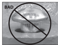
OVAL NECK OF BOLT NOT SEATED PROPERLY
