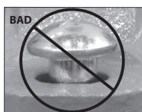
OVAL NECK OF BOLT NOT SEATED PROPERLY
