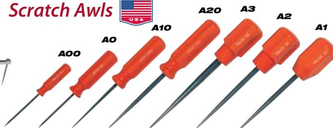
Use to scribe lines on metal, plastic and a variety of other materials. Pierce holes in wood, plastic, leather, - even light gauge metal. Blades are high carbon, alloy tool steel fully polished to resist rust. Blade tapers to a fine point and may be resharpened many times. Easy-to-spot orange handles are shock and shatter resistant. Shallow fluted handles with large end bearing surface provide a sure, comfortable grip. User has choice of large diameter or regular grip handles.
