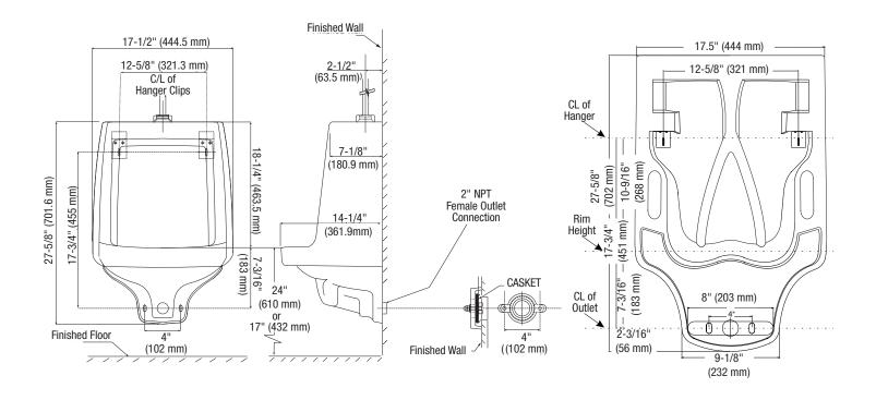
All dimensions and specifications are nominal and may vary: Dimensions of 8" and greater have a tolerance of +/-3%. Dimensions less than 8" have a tolerance of +/-5%.
