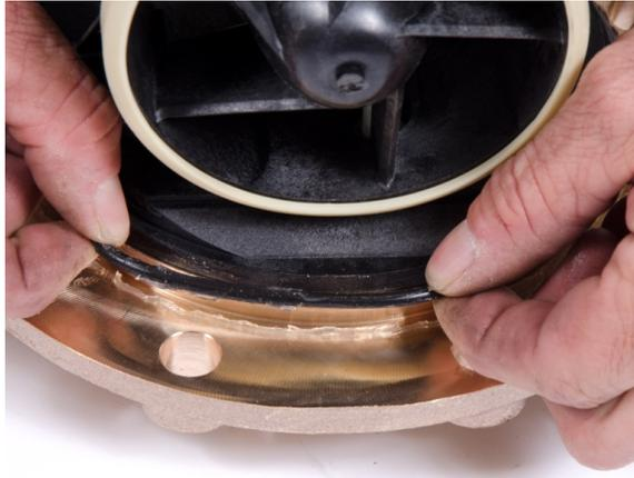
Figure 12 – Inspecting the O-Ring
