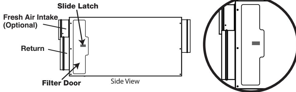
Step 2: Remove the filter by gently pulling it straight out of the unit. Insert new filter by gently pushing it into the unit. Make sure the AIR FLOW arrow on the filter is pointing into the unit.
