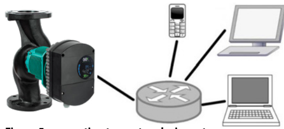
Figure 5: connecting to a network via router
