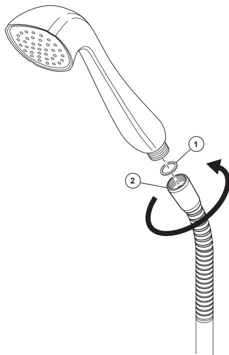
**Connect tapered end of hose to hand shower:** Seat the washer (1) firmly into the hose nut (2). Carefully align the thread of the tapered end of the hose (2) directly to the hand shower. **Hand Tighten—do not use a wrench or pliers.** Then place the hand shower into the wall mount holder.
