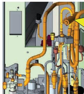
This is the position of the 4-way valve. Do not touch it directly with your hands. There is hot refrigerant at the discharge pipe, so be careful not to be scalded.
