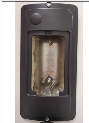
Figure 19 - Sensor Clip Installed on the Lower Stud
