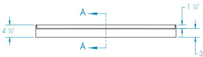
**FEATURES** Dimensional Tolerance  $\pm \frac{3}{8}$ ". Dimensions needed for site preparation should be measured from the unit. Aquatic assumes no responsibility for preparatory work.
