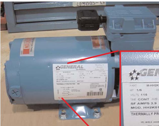
For Single Phase Oil-Less Compressors with All Other motors (as shown left) see page 3 or 4, depending on model number for wiring instructions.
