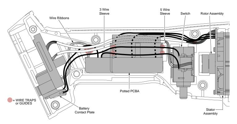
AS AN AID TO REASSEMBLY, TAKE NOTICE OF WIRE ROUTING AND POSITION IN WIRE GUIDES AND TRAPS WHILE DISMANTLING TOOL.
