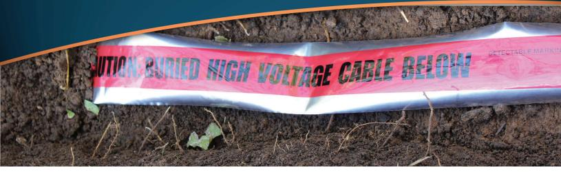
Presco Detectable Underground Warning Tape is used for accurately locating and preventing damage to valuable underground utility installations. It has an aluminum backing to make underground assets easy to find using a non-ferrous locator. Properly installed, this tape helps avoid catastrophically inaccurate digging when locating utilities such as electrical lines, gas pipes and communication cables.
