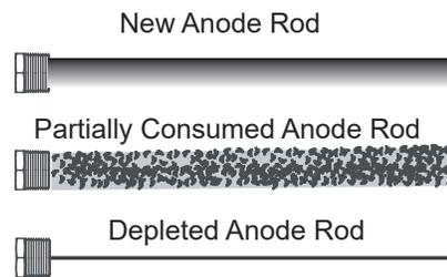
Figure 4. Anode Depletion
