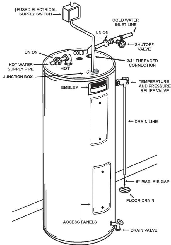
† OVER CURRENT PROTECTION MUST BE SUPPLIED IN WATER HEATER CIRCUIT. CONSULT LOCAL CODE OR CURRENT EDITION OF NEC FOR PROPER INSTALLATION.
