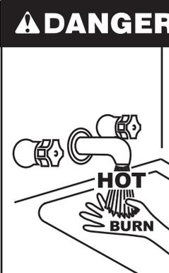
Water temperature over 125°F (52°C) can cause severe burns instantly resulting in severe injury or death.
