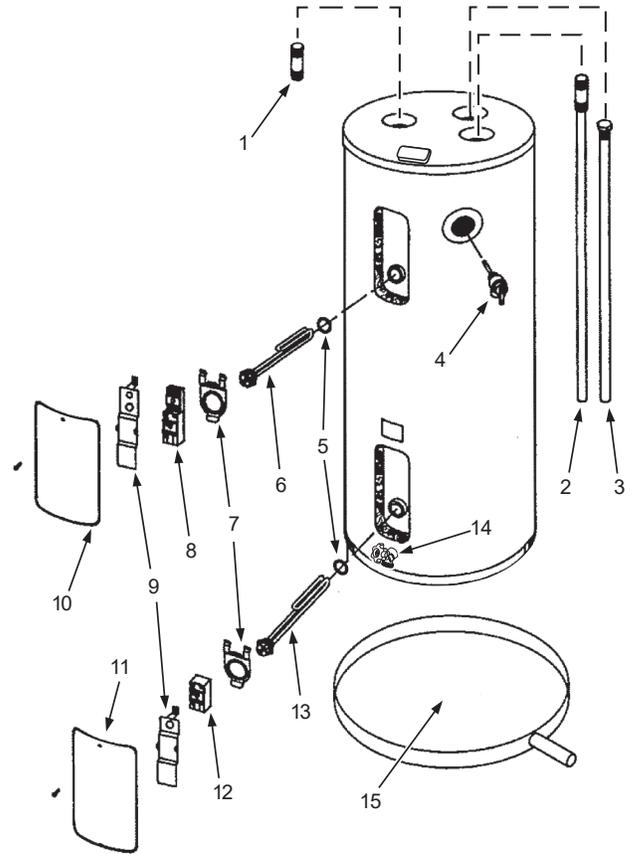
**Figure 7. Repair Parts**
