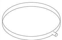
Install suitable drain pans under water heaters to prevent damage due to leakage. See *Locating the Water Heater* (page 11).
