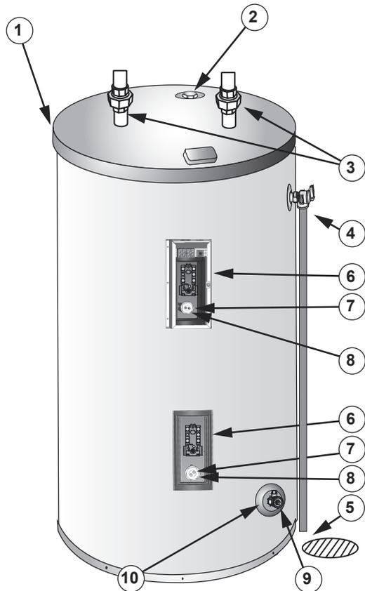
Figure 8. Leakage Checkpoints
