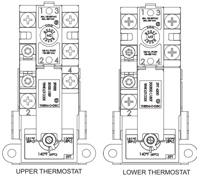
Figure 3. Thermostat Controls
