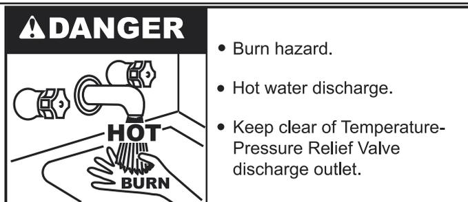
It is recommended that the Temperature-Pressure Relief Valve should be checked to ensure that it is in operating condition every 6 months.
