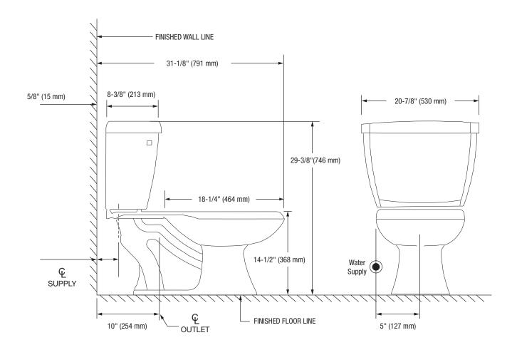
Note: All dimensions and specifications are nominal and may vary: Dimensions of 8" and greater have a tolerance of +3%. Dimensions less than 8" have a tolerance of +5%.
