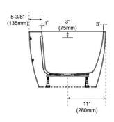
Dimensions of fixtures are nominal and may vary within the range of tolerance established by CSA B45.5-17/IAPMO Z124-2017.
