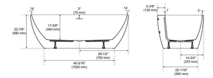
Dimensions of fixtures are nominal and may vary within the range of tolerance established by CSA B45.5-17/IAPMO Z124-2017.
