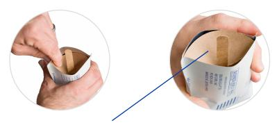
Radon gas easily passes through the draft-shield
