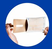
Seal the Test Kit to ensure no radon escapes. Fold flap to expose adhesive strip.
