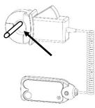
Depress the clamp lever and place the CT around the hot or neutral wire where AC current is to be measured. Make sure the clamp jaws are fully closed for best accuracy. If there is a ferrous metal surface near the placement of the clamp, the magnet on the bottom of the radio module can be attached to the surface for a more secure connection.
