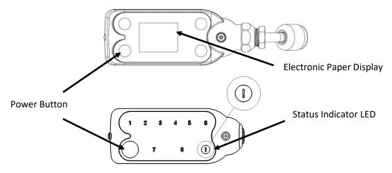
When using the YJACK PATH<sup>®</sup>, numeric LEDs 1-8 will illuminate to indicate the number of YJACK<sup>®</sup> and P51-870 TITAN<sup>®</sup> devices within range.
