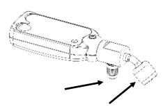
Remove the red plug from the brass quick coupler nut. Make sure the pressure transducer has been zeroed (this will be covered in more detail later) and attach the device directly to the system low-side or high-side service port. A 5/16" adapter (19121 straight or 19221 90 degree) can be used for systems with 5/16" connections. The integrated charging port on the back of the device can be connected to a charging hose for adjustment of system charge while continuing to monitor system pressure.
