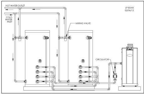
Figure 11 - Dual Purpose Application with Two Water Heaters
