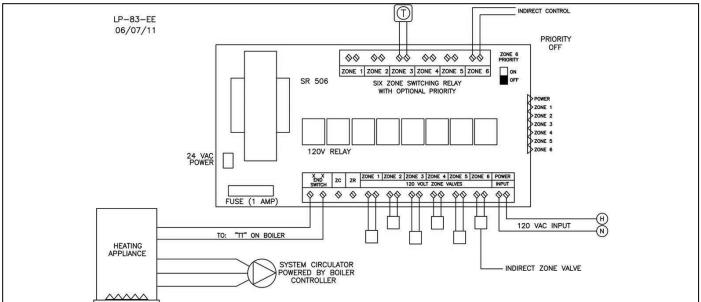
Figure 17 - Wiring with Zone Valves
