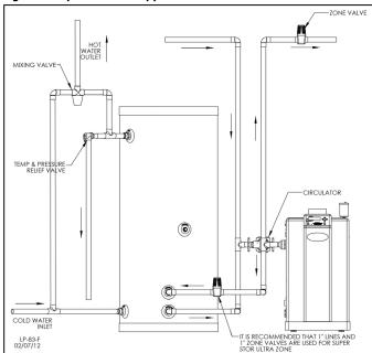
Figure 5 - Installation with High Efficiency Boiler
