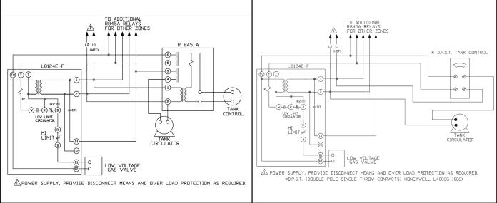
Figure 20 - Zoning with Circulators Using L8124 A, C, and R845A Relay
