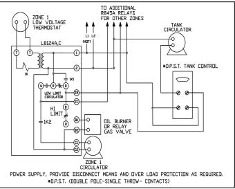
Figure 26 - Zoning with Circulators Using L8124 E-F, and DPST - No Relay Required
