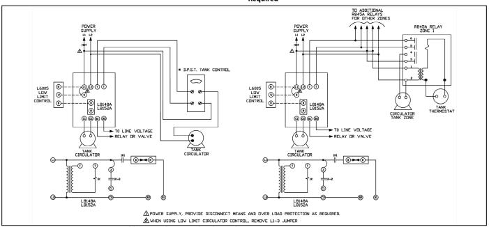
Figure 22 - Using L8148A or L8152A Cold Start Boiler Control with Circulators
