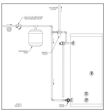
Figure 4 - Expansion Tank Application
