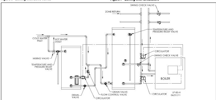
Figure 8 - Installation with Storage Tank
