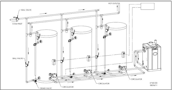
Figure 15 - Multiple Tank Installation
