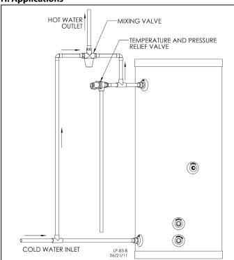
Figure 3 - Mixing Valve Installation
