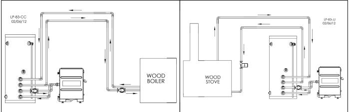
Figure 9 - Dual Purpose Application with Wood Boiler
