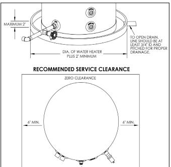
Figure 1 - Drain Pan Installation and Recommended Service Clearances
