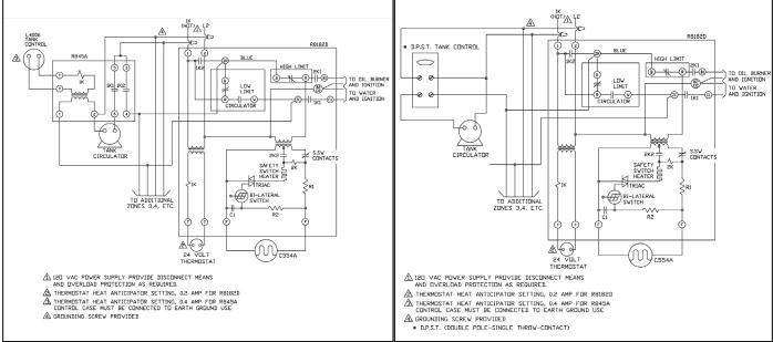
Figure 23 - Zoning with Circulators - R8182D and R845A Relay
