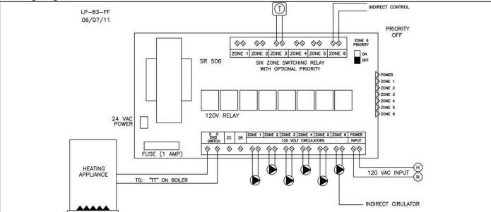
Figure 16 - Wiring with Circulators
