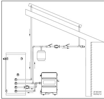
Figure 12 - Dual Purpose Application with Solar Panel
