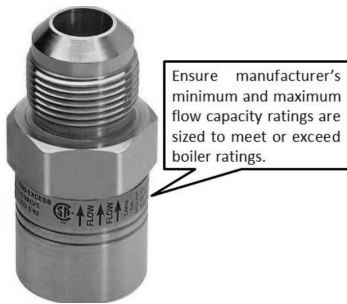
Figure 46 - Excess Flow Valve (EFV)
