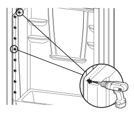
Fasten flanges along top of left side walls with fasteners of choice (see Pre-Installation Planning #12) into each corresponding stud. Fasten side (vertical) flanges to side studs 8" (200mm) on center. **NOTE:** Finish caulking is not required, however, if using caulk, weep channel must be remain clear of obstruction to allow for proper drainage of the unit.
