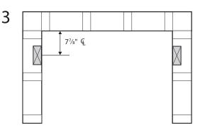
Pre-install unit to ensure framing pocket is plumb, square and a level installation can be achieved (see steps 3 through 9).
