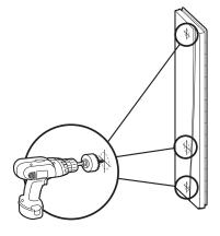
Using a hole saw (fine tooth or abrasive grit cutting edge), make necessary openings for filler and valves, drilling from inside (smooth side) out.
