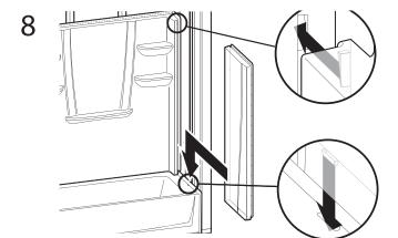
Slide right side wall into position. Be sure locking mechanism is engaged.
