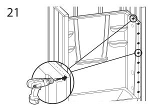
Fastened flanges along top of right side wall with fasteners of choice. (See Pre-Installation Planning #12) into each corresponding stud. Fasten side (vertical) flanges to side studs 8" (200mm) on center.
