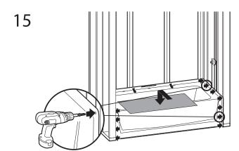
Pre-drill horizontal flanges along top of base section and fasten into each corresponding stud. Pre-drill both (vertical) side flanges and fasten to side studs 8" (200mm) on center. Place cardboard to protect surface.
