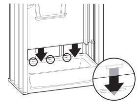
Lift and place back wall, making sure locking tab is engaged.
