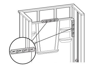
Level back wall vertically. Shim if necessary.
