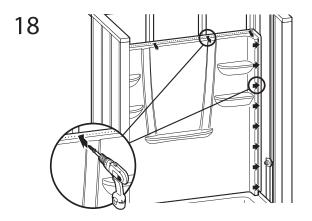
Fasten flanges along top of back wall with fasteners of choice (see Per-Installation Planning #12) into each corresponding stud. Pre-drill both (vertical) side flanges and nail fasten to side studs 8" (200mm) on center.
