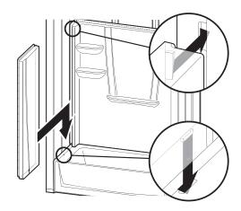
Slide left side wall into position. Be sure locking mechanism is engaged.
