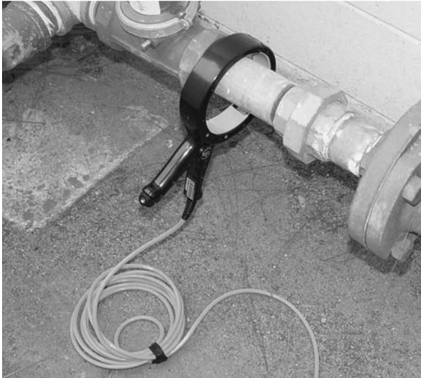
Figure 4 – Example: Attaching The Inductive Clamp
