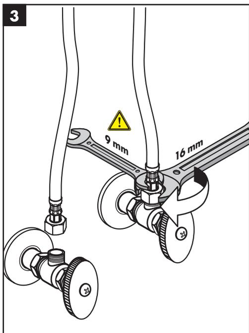
Connect the hot and cold supply hoses to the stops.
