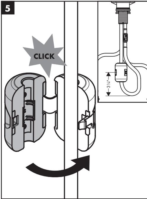
Install the hose weight 3 1/4" from the bottom of the hose.
