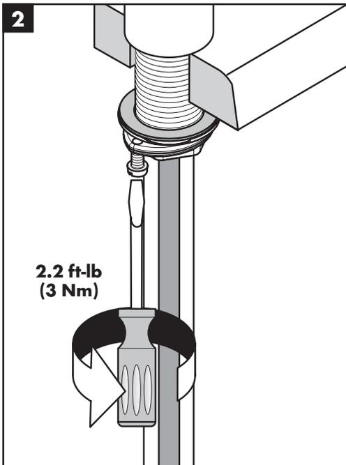
Tighten the mounting nut.
