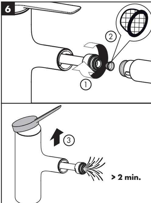
Remove the handspray. Remove the filter screen.
