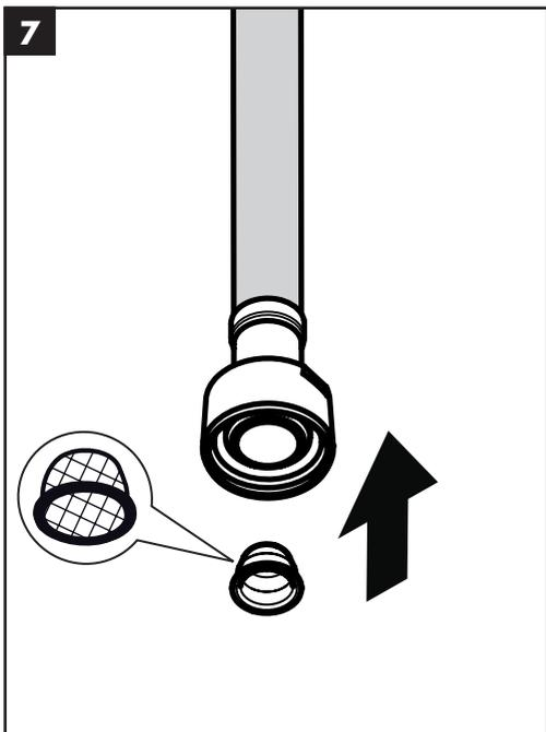
Install the filter in the handspray hose.
