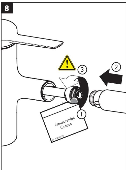
Lightly lubricate the hose o-ring.
