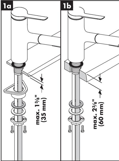
Place the faucet and sealing ring on the mounting surface. Install the support, friction washer, metal washer, and mounting nut.
