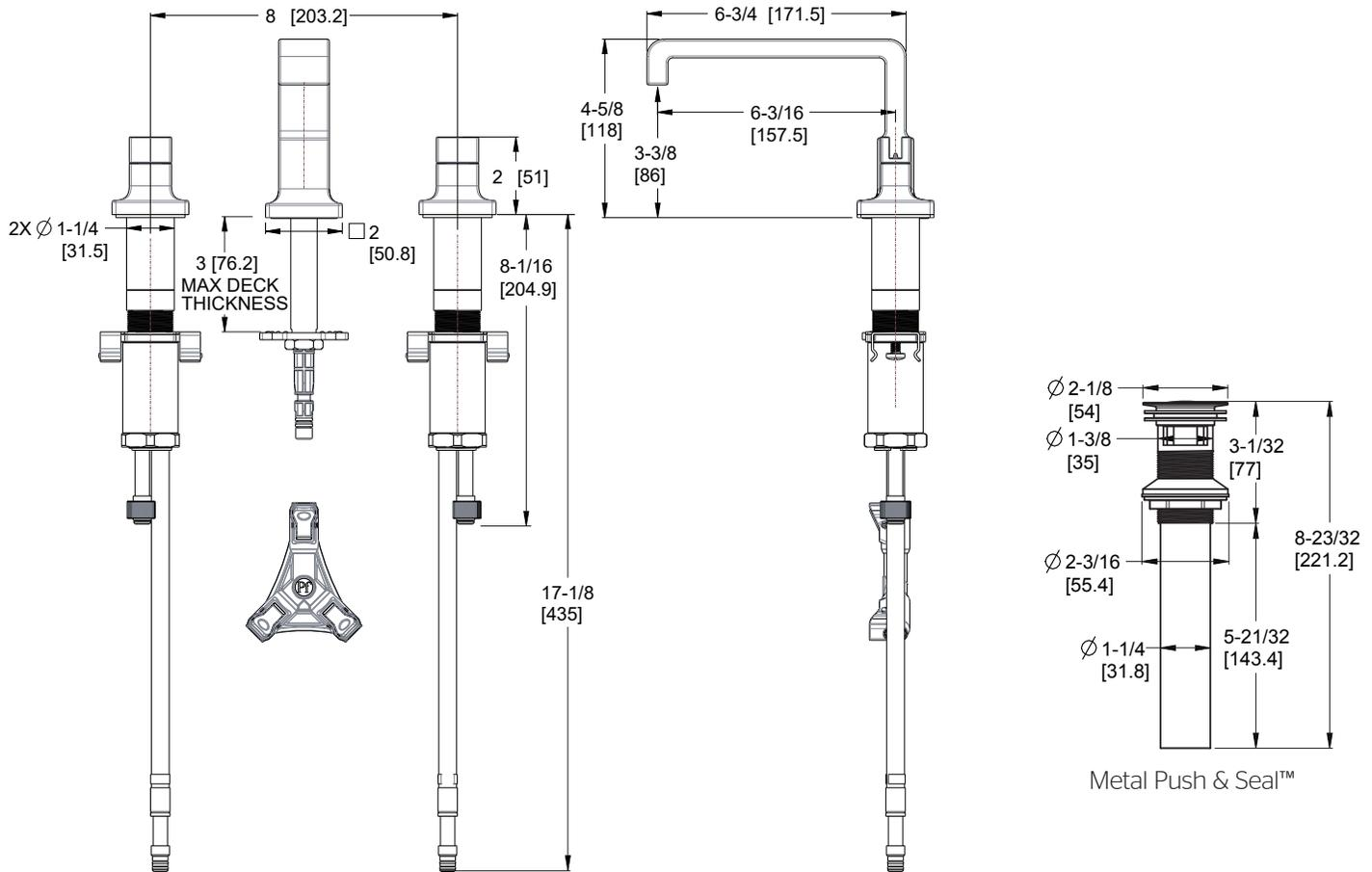
$\varnothing$ 1-1/4 Min to  $\varnothing$ 1-1/2 Max. Deck Hole Openings
