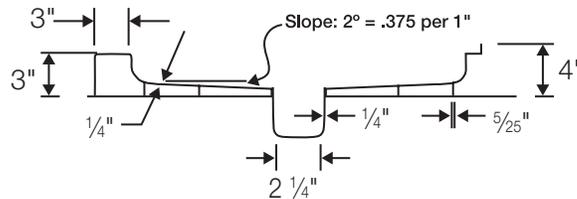
**FEATURES** Dimensional Tolerance  $\pm 1/4"$ . Dimensions needed for site preparation should be measured from the unit. American Bath Group assumes no responsibility for preparatory work.
