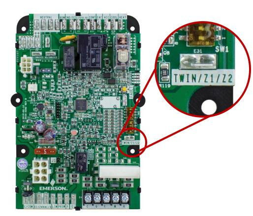
click to See If both Boards are not powered a Twinning fault of 6 red flashes occurs.
