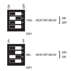
A screwdriver can be used to change settings through protective Dipswitch cover.
