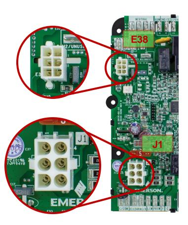
The ST9120 replacement does not require any additional wiring harnesses.
