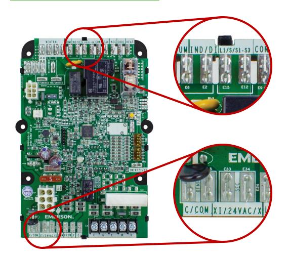
On some Terminals multiple identifiers are Silkscreened on the board. All cross-over boards are identified and referenced on each Terminal, making it easy for correct placement of wires.
