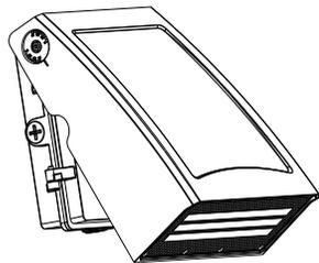
10. Fixtures with photocell should be mounted at least 48" from all sides to avoid reflection of light back onto Photocell, causing the Photocell to malfunction or flicker.
