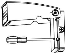
3. Punch out appropriate knockouts on the mounting box, and apply the adhesive gasket to the back surface of mounting box, mount the box to J-box with screws.
