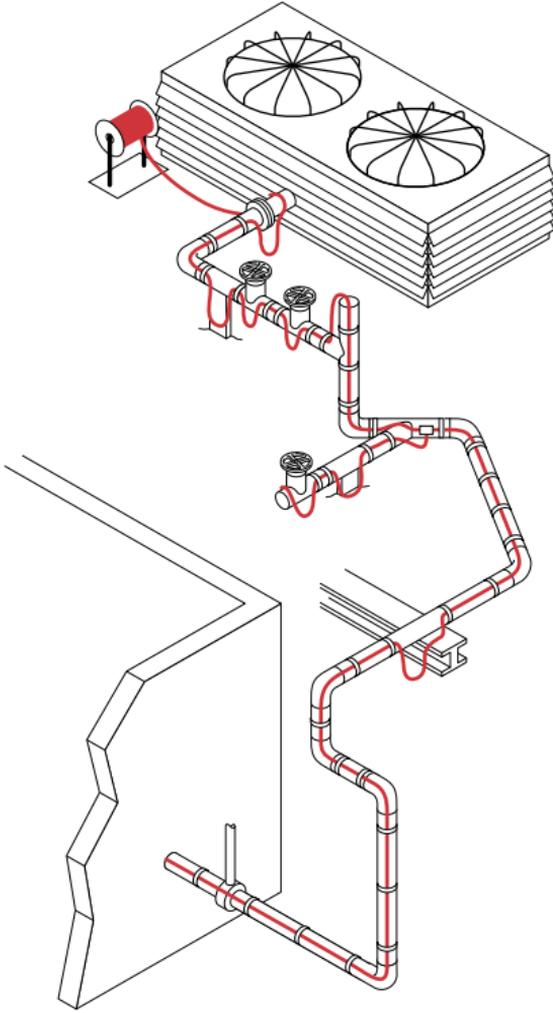
**Figure 3: Attaching the heating cable**
