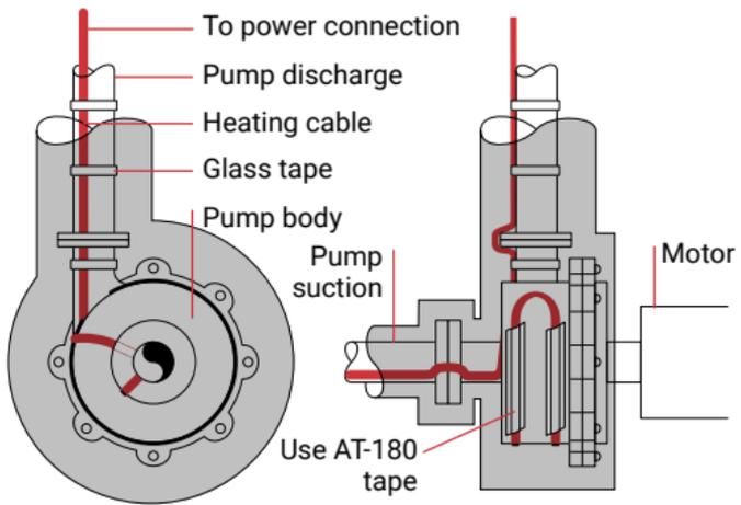
**Figure 13: Split case centrifugal pump**
