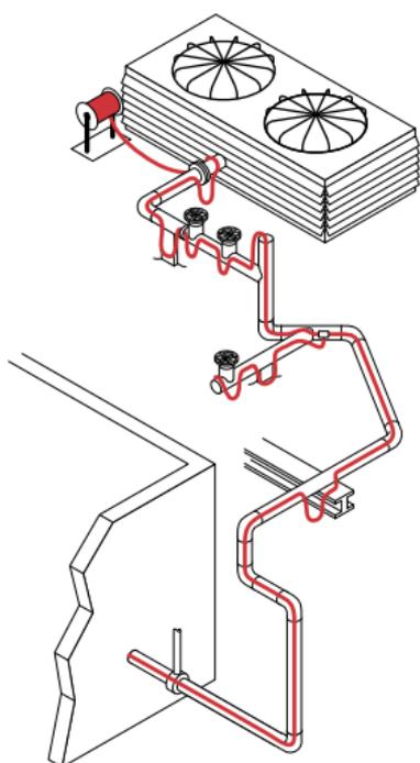
**Figure 2: Paying out the heating cable**
