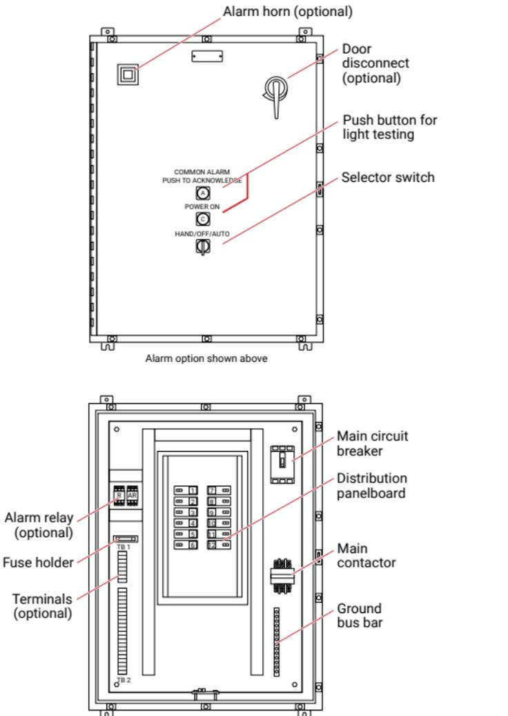
**Figure 26: HTPG power distribution panel**
