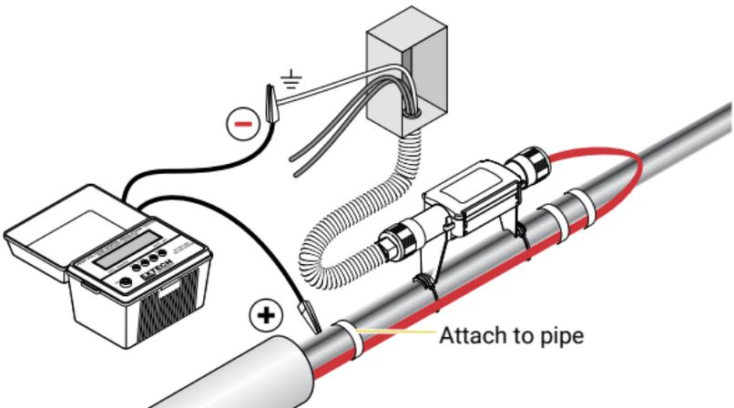
Figure 28: Insulation resistance test
