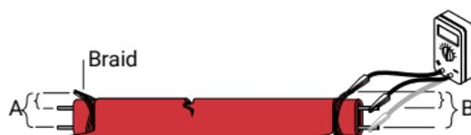
**Figure 32: Low resistance ground-fault test**
