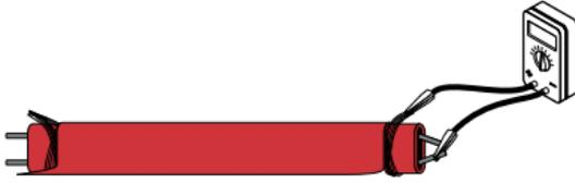
**Figure 29: Capacitance test**
