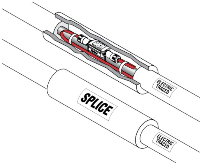
**Figure 22: Installing connection kits below insulation**
