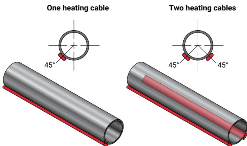
Figure 7: Positioning the heating cable
