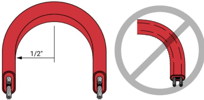
**Figure 9: Bending technique**
