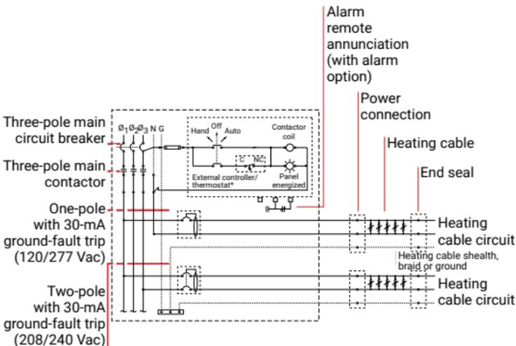
**Figure 27: HTPG schematic**
