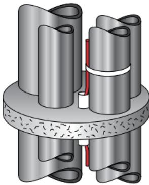
**Figure 6: Multiple pipe floor penetration**
