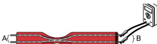
**Figure 31: Heating cable resistance measurement test**
