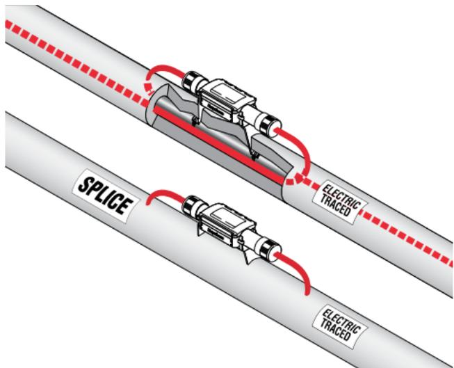
**Figure 23: Installing connection kits above insulation**
