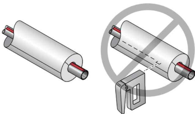
**Figure 21: Sealing the insulation seam**
