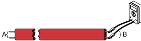
**Figure 33: Heating cable resistance measurement**
