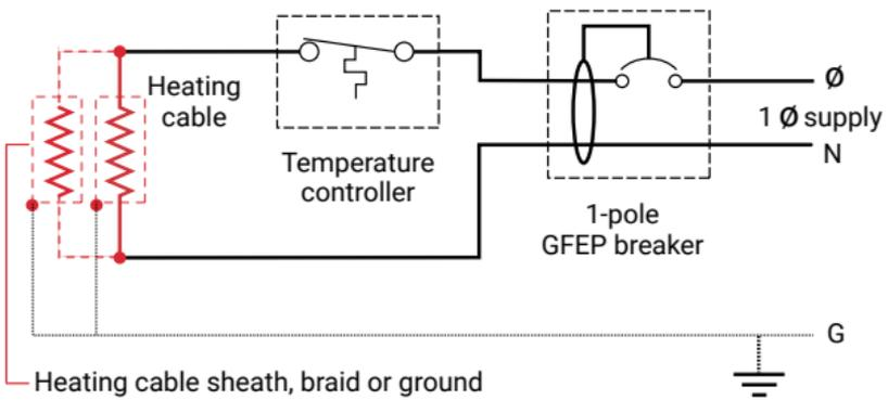
Figure 24: Single circuit control
