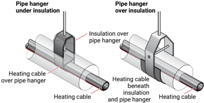
**Figure 4: Pipe hanger with heating cable**
