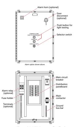
Figure 26: HTPG power distribution panel
