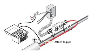
Figure 28: Insulation resistance test
