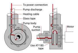
Figure 13: Split case centrifugal pump
