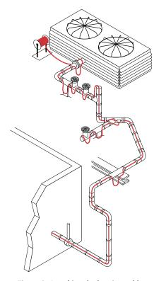
Figure 3: Attaching the heating cable
