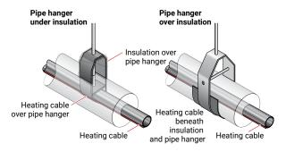
Figure 4: Pipe hanger with heating cable
