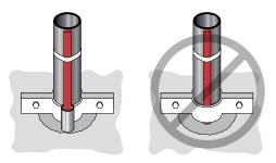
Figure 5: Single pipe floor penetration
