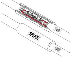
Figure 22: Installing connection kits below insulation
