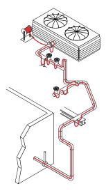
Figure 2: Paying out the heating cable
