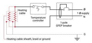
Figure 24: Single circuit control
