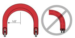
Figure 9: Bending technique
