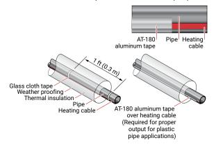
Figure 8: Attaching the heating cable
