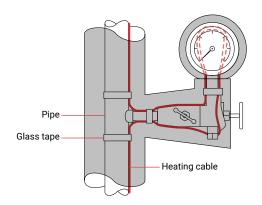
Figure 12: Pressure gauge
