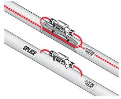
Figure 23: Installing connection kits above insulation
