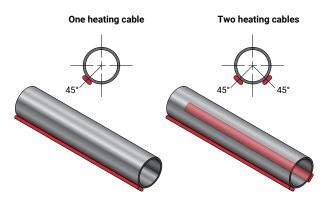
Figure 7: Positioning the heating cable
