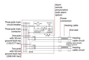
Figure 27: HTPG schematic
