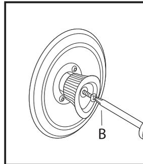
4. With spacer ring (D) in place, replace with new handle.
