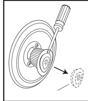
3. Unthread screw (B) to remove handle (C).
