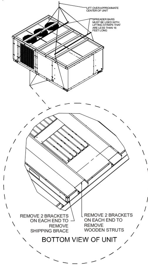
3. Lift unit per the "Rigging Details" section of this manual, observing all warnings and cautions. When unit is lifted, boards and shipping brace will drop if screws have been removed. To avoid injury, STAND CLEAR.
