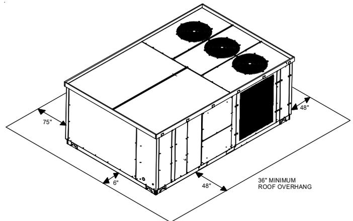
*\*In situations that have multiple units, a 48" minimum clearance is required between the condenser coils.*
