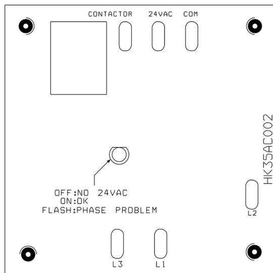
**Fig. 7 – 3-Phase Monitor Control**
