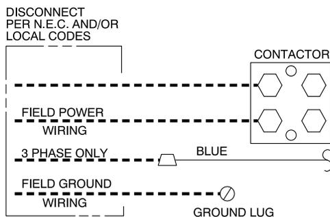
**Fig. 6 – Line Connections**
