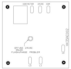
Fig. 7 – 3-Phase Monitor Control (Applies to 3-Phase Units Only)
