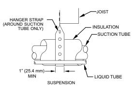
Fig. 1 – Piping Installation
