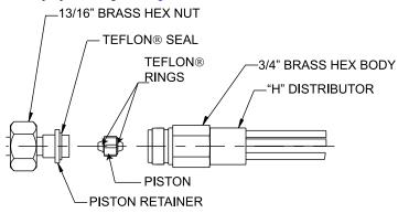
Fig. 5 - Indoor (Cooling) Piston
