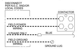
Fig. 6 – Line Connections
