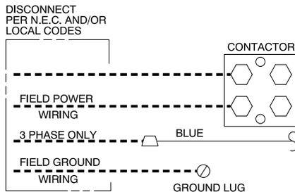
Fig. 5 – Line Power Connections
